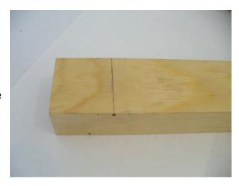
Next, make marks 9/16" in from each side of the edge of the car at the axle hole. These locations are where the inspection holes will be centered.
