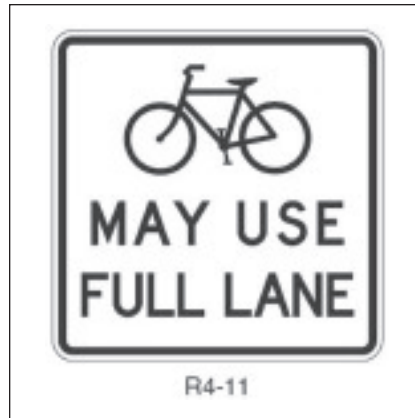
Figure 3. A “Bicycles May Use Full Lane” regulatory sign is for optional use where a travel lane is too narrow for bicycles and motor vehicles to operate side by side in the same lane.
