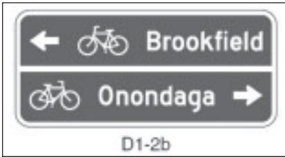
Figure 1. The new MUTCD is proposing an innovative system of bicycle guide signing that can provide considerably more comprehensive guidance than the simple “bike route.”
