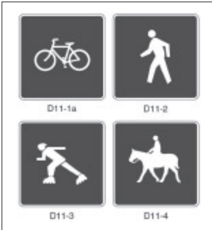
Figure 2. Another proposed signing improvement is to add a set of mode-specific informational signs that can be installed on shared-use path corridors where separate travelways are provided for different user types.
